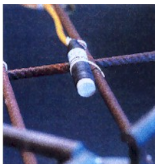
Figure C17. Photograph of the Embedded Reference Electrode Produced by ERE
