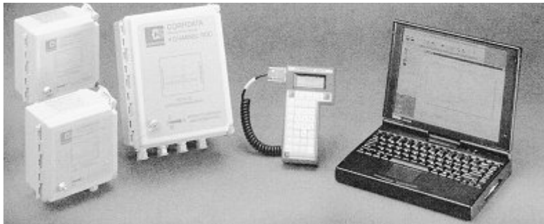
Figure C26. Remote data Collection System for Corratr Probe
