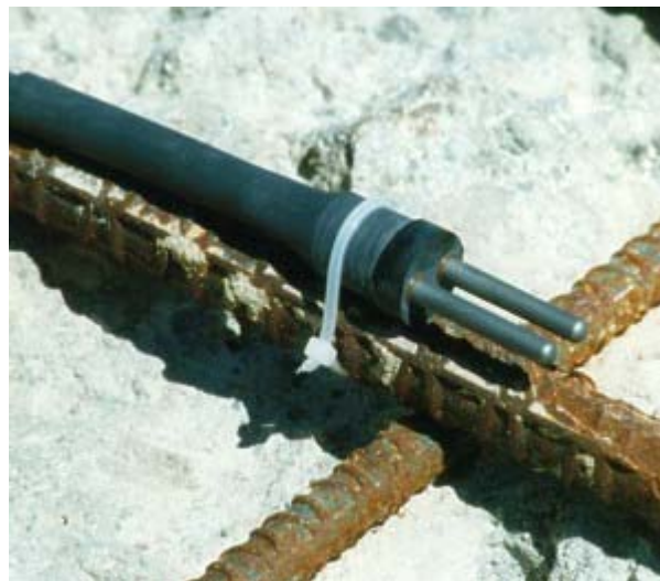
Figure C25. Embeddable LPR Probe (Model 800/800T Corratr Probe)
