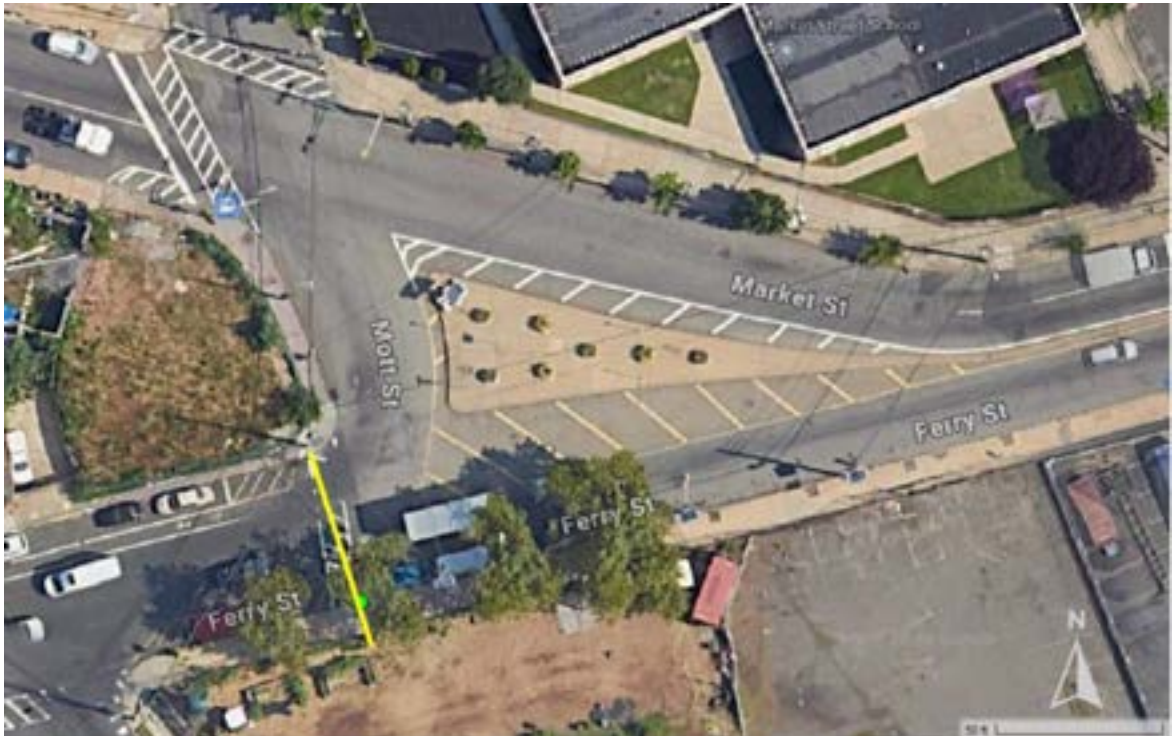
Figure 13 a) Water flow, depth, and speed at the Down Bottom Farms Traffic Triangle site from HEC-RAS simulation. b) Aerial photo of the site indicating the reference line (yellow line) where flow was extracted, and the reference point (green point) where depth and speed were measured.
