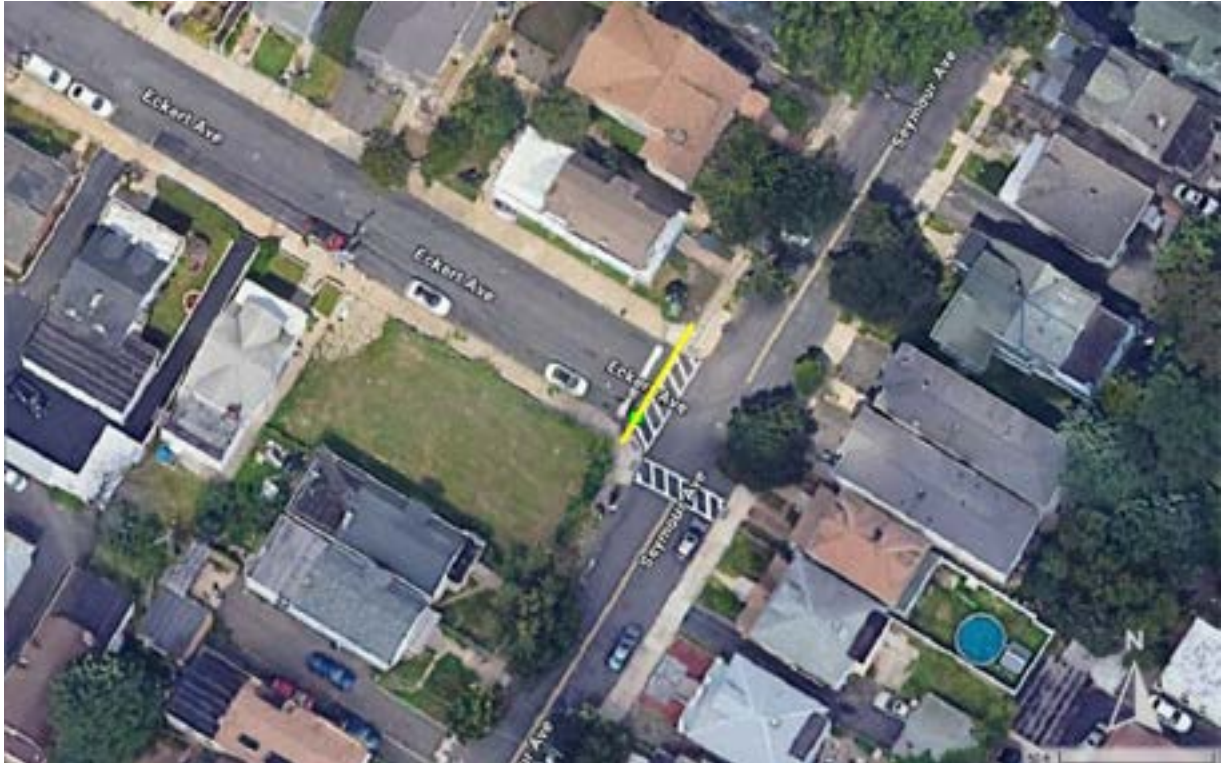
Figure 9 a) Water flow, depth, and speed at the Art of Survival Garden site from HEC-RAS simulation. b) Aerial photo of the site indicating the reference line (yellow line) where flow was extracted, and the reference point (green point) where depth and speed were measured.
