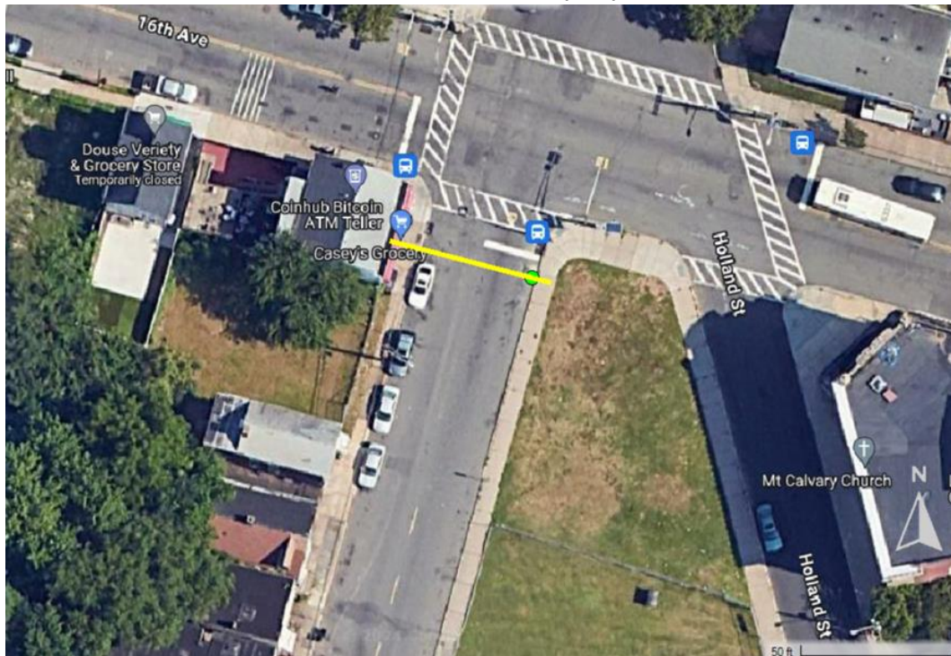
Figure 12 a) Water flow, depth, and speed at the Harriet Tubman Elementary School site from HEC-RAS simulation. b) Aerial photo of the site indicating the reference line (yellow line) where flow was extracted, and the reference point (green point) where depth and speed were measured.
