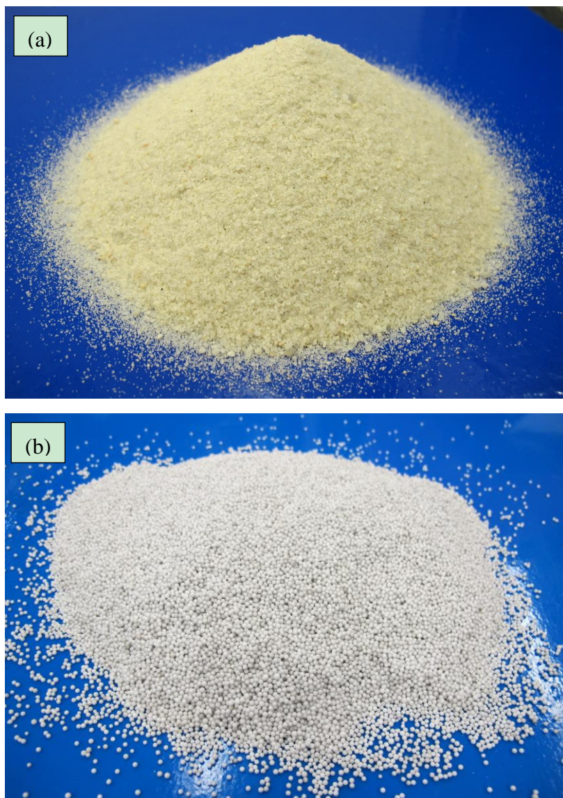
Figure 7. (a) Natural screened and washed sand; and (b) Foamed polymer particles
