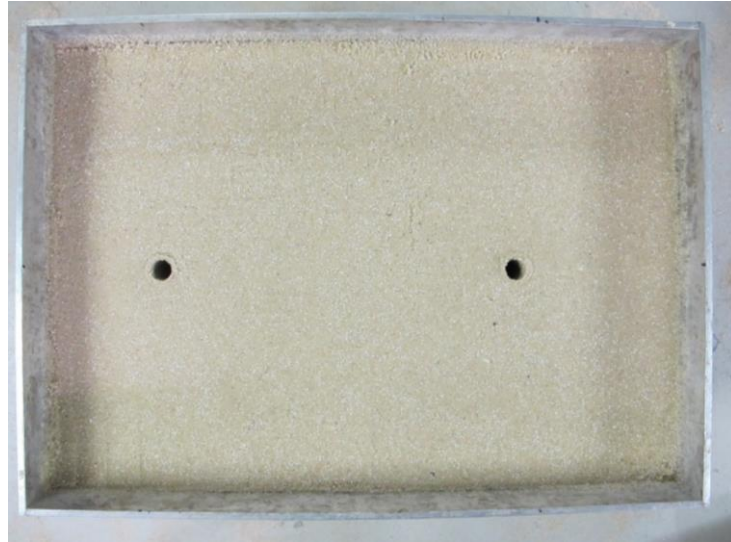
Figure 9. A prepared composite sample with mixed sand and foaming particles.
