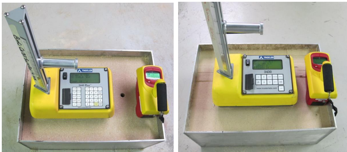
Figure 11. Nuclear gauge devices: (a) Cs-137 source; and (b) Am-241: Be source.
