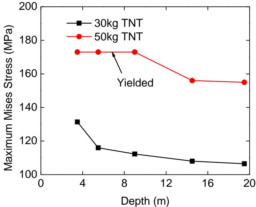
Fig.6 Effects of burial depth on lining stress
