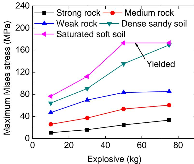
Fig. 4 Effects of explosive weight on lining stress
