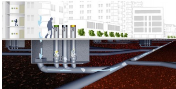
A pneumatic schematic. Envac.
